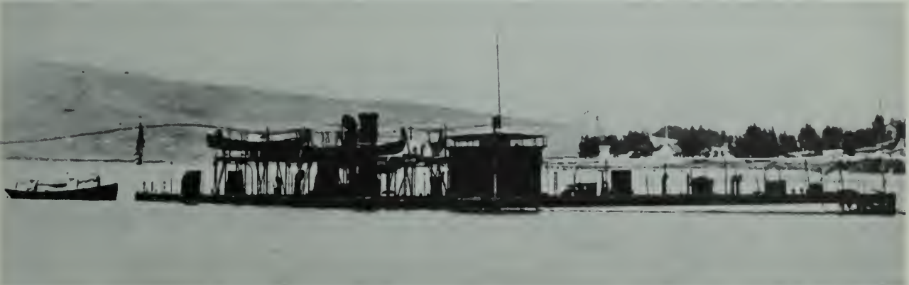
U.S. Monitor Camanche as she appeared in 1898—The Civil War monitors which were not fully rebuilt but which remained on the Navy List received additional deck ventilators and a light hurricane deck over the years, the once long and low clean lines becoming cluttered and ugly.
